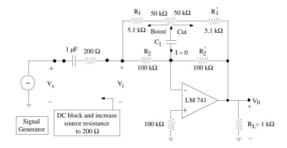
The corner frequency, defined for max. boost/cut positions, is where the transfer function deviates from the flat response by  $\pm 3$  dB. It is given by:
