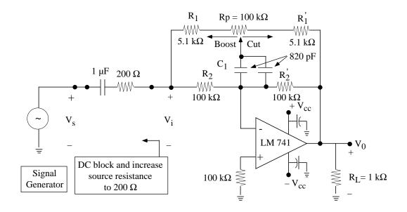
At high frequencies, when the C<sub>1</sub> (2 x 820 pF) behaves as a short-circuit, the circuit becomes:
