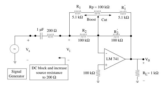
If the 100 k $\Omega$  potentiometer is set at maximum boost, the gain becomes:
